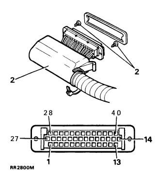
Pins 1 to 13 bottom row. Pins 14 to 27 centre row. Pins 28 to 40 top row.
