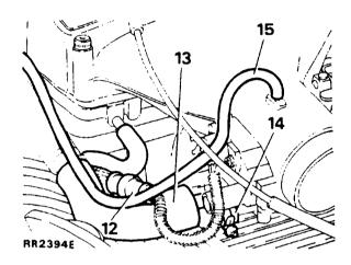
16. Release the two screws and remove the potentiometer.
