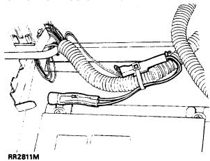
The 14CUX system is used in various markets, but a common ECU is used. To suit individual market requirements a tune select resistor is connected across pins 5 and 27 of the ECU.
