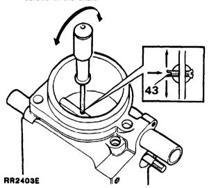
44. Pre-grease a new air seal with Admax L3 or Energrease LS3. Fit the seal pushing it down the shaft and into the counterbore until the seal is 6.0 mm (0.236 in) below the face of the plenum chamber.
