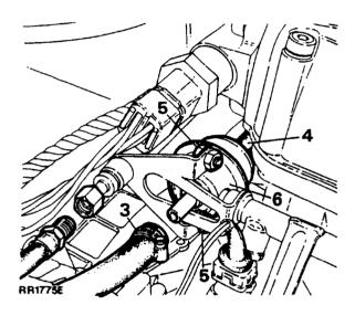
NOTE: If the original regulator is being refitted, fit a NEW 'O' ring to the fuel inlet pipe.
