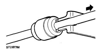
NOTE: To disconnect the 'speedfit' connector, forked end into the two slots of the connector as shown in the illustation above. Press down on the collet and simultaneously pull the pipe from the connector. Special tool LST 144 is available for this operation.
