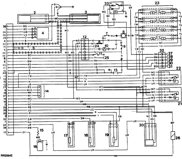
FUEL INJECTION - Circuit Diagram - 1989 Model Year
