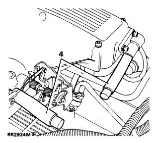
5. Start the engine and check that the idle speed is within the limits specified in Section 05 -Engine Tuning Data.
