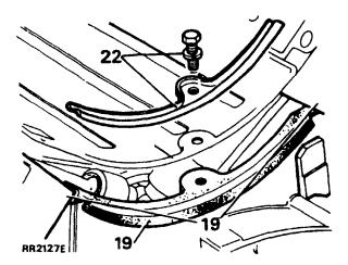
Lightly apply 'Hylomar' sealant around the outside of the water passage openings on the cylinder heads, manifold gasket and intake manifold.
