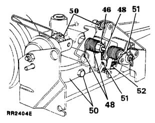
NOTE: If new throttle levers have been fitted the minimum throttle setting of the disc must be checked to ensure that it is SO" to the bore.
