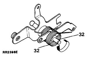
33. Wind a new spring onto the countershaft assembly noting that the small hooked end of the spring is wound on first.
