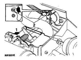
NOTE: Check the clearance between the cruise control actuator link and throttle lever (see Cruise Control Actuator Setting-Section 19, Page 47).
