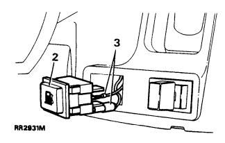
Remove the release button from the shroud and disconnect the two wiring connectors. Ensure that the wires protrude through the shroud to facilitate reassembly.
