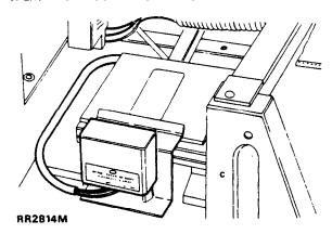
1990 model year vehicles have a fault code display unit which is located underneath the right hand front seat, adjacent to the EFI ECU. The unit will display the relevant fault code, in addition to the EFI warning light being illuminated.
