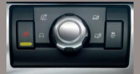
**TERRAIN RESPONSE®** Land Rover's patented Terrain Response® system\* adds to Freelander 2's breadth of capability. Any of the four programmes — general driving, grass/gravel/snow, mud and ruts, or sand — can be easily selected by simply turning the rotary control. In addition all vehicles with Terrain Response® are also fitted with Hill Descent Control\* and Land Rover's Gradient Release Control systems\*.
