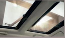
PANORAMIC SUNROOF The optional panoramic sunroof with a fixed rear section and electric tilting/sliding front section – adds to the feeling of lightness and airiness within the cabin. The glass is specially formulated to filter the sun's infrared rays, providing light without unpleasant heat. Both sections also include a convenient blind
