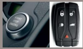
REMOTE CONTROL AND START/STOP BUTTON The remote control includes the following functions: locking and unlocking of the doors and tailgate, a 30 second courtesy headlamp delay and activation of panic alarm. In order to start the car the remote has to be docked into the facia and the correct procedure followed using the Start/Stop button.
