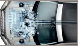
PERFORMANCE WITH REFINEMENT. The 2.2 litre turbodiesel engines, now available in power outputs of 150PS and 190PS, come with common-rail diesel technology which aids economy and refinement and a Variable Nozzle turbocharger helping to deliver exceptional torque.
