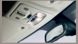
**CONVENIENCE FEATURES** Life with Freelander 2 is so practical thanks to thoughtful technology. Available features include: An electrochromatic rear view mirror for automatically minimising the dazzle of headlamps at night. Rain sensing wipers and twin map lights conveniently located in the roof console above the rear view mirror.
