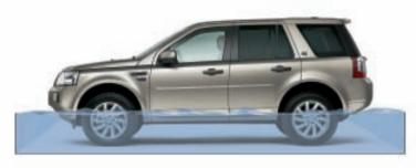
Wading Depth Maximum wading depth 500mm
