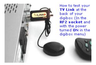
Most faults are caused by badly fitted connectors and short circuits. This causes the problems as power does not reach the link along the Coaxial vable.
