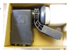
1. Remove the existing arm off the LNB
