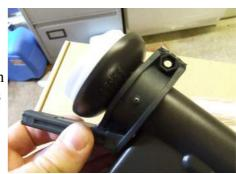
5. Insert the Nut + Bolt and tighten. This is now suitable for a <u>Type 1</u> dish.
