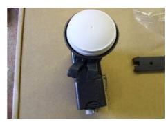
6. Add the insert as shown (there is a notch out of the 'top' side half of the insert) for dishes that are 'Type 2' (This is most recent dishes)
