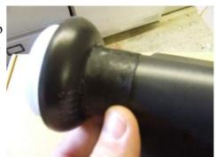
4. Position the new arm so that the plastic nobble lines up with the number 3 on the side of the LNB
