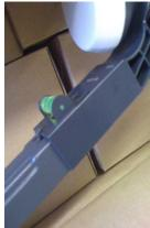
Place the edge of the LNB so that it rests under the edge of the protruding tab.
