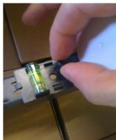
To finish, simply push the plastic insert (snap it off the LNB if it is still attached) into the hole.
