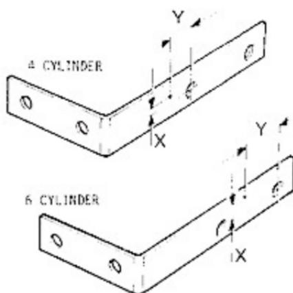
4 Remove the bracket, and from the pencil mark measure distances X and Y in relation to the fixing hole which is going to be used i.e. rear hole for four cylinder models and the front hole for six cylinder vehicles.
