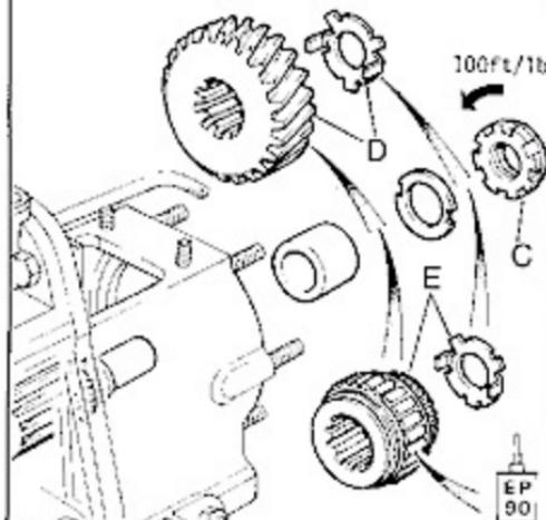
**9** Using special spanner 600300, remove mainshaft nut C. Withdraw lockwasher and gear D. Fit clutch sleeve and NEH lockwasher E, ensure that the distance piece and shim (if fitted) are re-assembled in the order shown. Tighten mainshaft nut and lock with washer.
