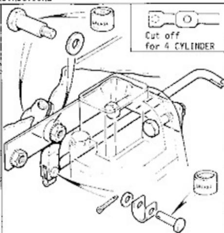
6 Assemble the link rod to the operating pivot and place in position. Refit the 'L' shaped bracket to the transfer box, and secure the operating pivot to the bracket.
