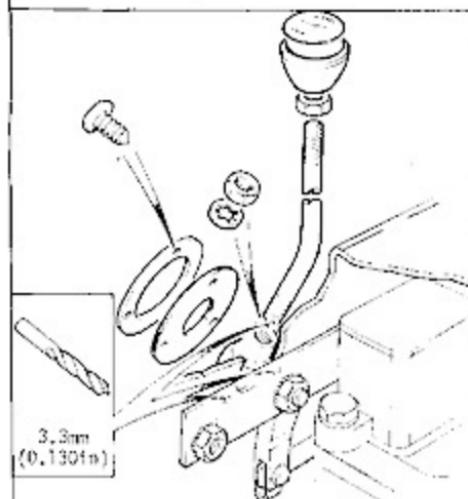
7 Position the rubber grommet and sealing plate over the operating pivot, drill three holes and secure with self tapping screws. Assemble the operating lever and knob and fit to pivot.
