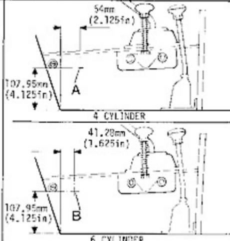
2 Mark and centre punch the transmission tunnel at point A or B whichever is appropriate.
