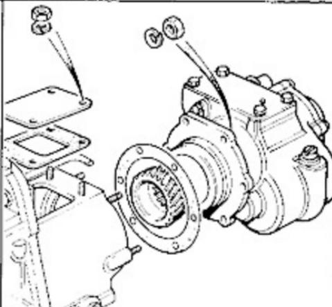
**10** Smear grease on both sides of gasket and fit to transfer box studs. On no account must the anti-scuff paste be wiped from the inside of the overdrive mainshaft. Offer overdrive into transfer gearbox (see special notes 11). Ensure the studs do not foul the overdrive casing and secure with original fixings. Refit cover and gasket to top of transfer box.
