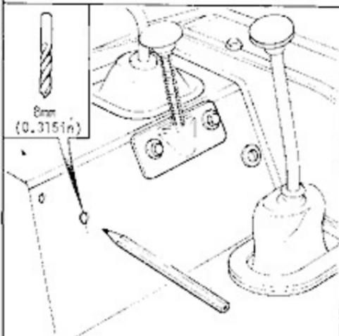
3 Drill a hole at point A or B and with a pencil through the hole, mark the bracket previously fitted.
