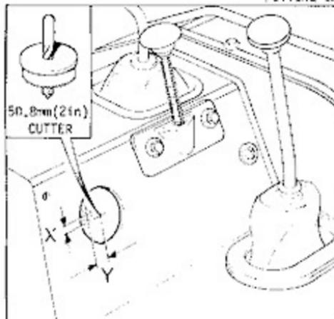
5 Transfer the measurements X and Y onto the transmission tunnel and where the two lines intersect, centre punch and cut a hole to the dimensions shown.
