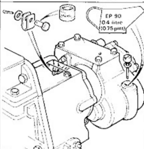
**12** Connect link rod to selector shaft. Fill unit with oil. Dipstick reading should be obtained by screwing fully into place. Refit centre seat panel, affix clutch warning label. Adjust the operating lever to a suitable position and road test operation of unit.
