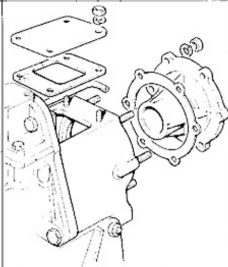
8 Remove rear bearing housing and top cover plate from transfer box.
