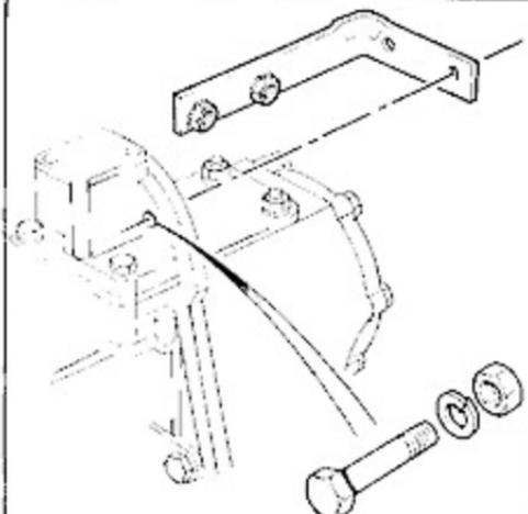
1 Remove centre seat panel. Fit the 'L' shaped bracket to the vertical bolting flange of the transfer box using the replacement fixings.
