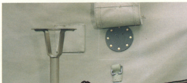
Aerial outlet and support brackets.
